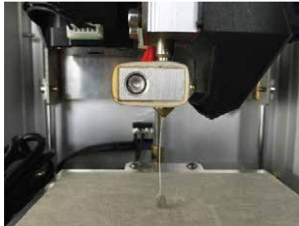
NOTE: The extruder cooling fan will come on anytime the extruder is above 50° and will turn off automatically when the extruder cools below 50°.
