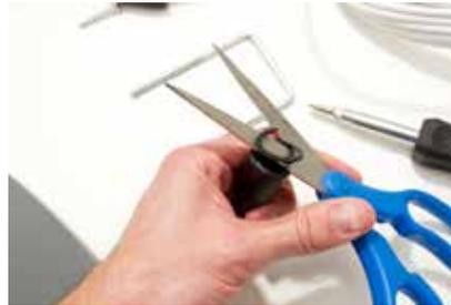
**Note:** You may need to trim a small section off the black jacket in order to more easily attach the coax cable to the antenna. Trim off a small section as shown above.
